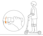
3. Put your other foot on the footrest to keep both feet stable. Press the throttle on right hand to speed up when you are balanced. Note, For your safety, the motor will not engage until the scooter reachs 1.8 mph (3 km/h).
